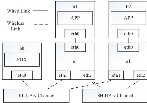
**Figure 2: A simple example of SDUWN. Two SDUWN nodes (h1-s1 and h2-s2) are equipped with both Short-range High-data-rate underwater acoustic modem and Long-range Low-data-rate underwater acoustic modem. The controller is on node h0 equipped with long-range low-data-rate underwater acoustic modem. The SDN switches on 2 nodes are configured by the POX running on h0. Application program is running on h1 and h2.**
