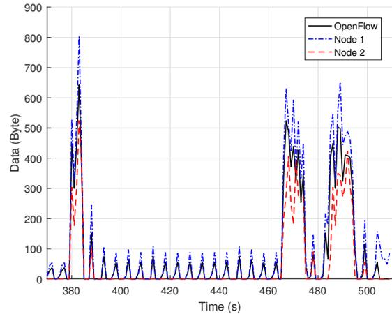
**Figure 4: 2-Node SDUWN example with ns-3 CSMA control plane channel. The delay for CSMA channel is 100ms.**
